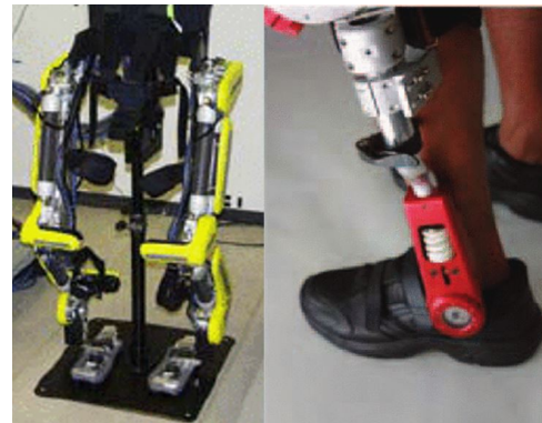
(c) Hybrid Actuators: Hybrid Motorized and Pneumatic Drive [81], Series Elastic Actuators [82]
