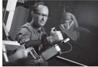
Fig. 3. Exoskeletal robotic arm used to control a dolphin simulation. Setup currently used in the SMARTS 2 trial (NCT02292251). The goal in this trial is to allow movement exploration in an immersive and engaging video game in order to boost motor recovery of the upper limb. Adapted from Krakauer and Carmichael (2017).
